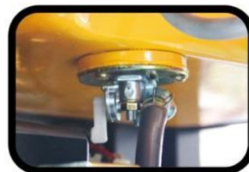
STEP 6. Turn the fuel switch on.
