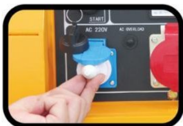
STEP 10. Connecting the load.
