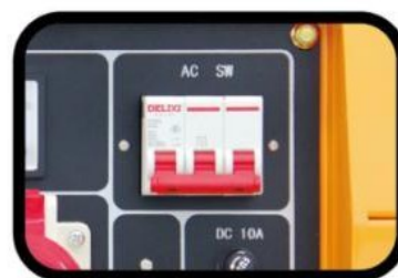
STEP 3. Turn the circuit breaker off.
