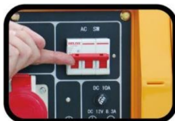
STEP 11. Turn the circuit breaker on.
