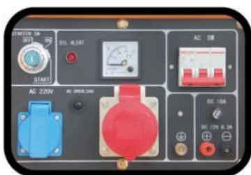
STEP 1. Disconnect any load.
