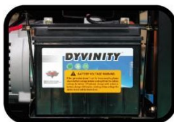
STEP 2. Connect the battery before starting.
