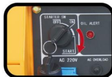
STEP 9. Turn the key switch to "start" position to start the engine directly.
